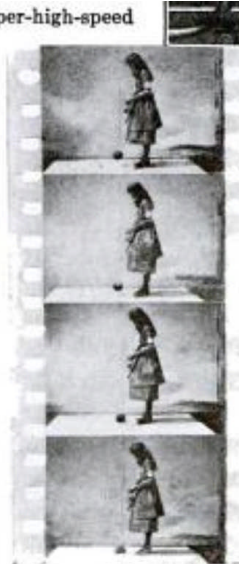
Movie film; showing how a rubber ball flattens at instant of impact
